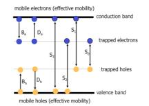
Figure 1: Schematic representation of the charge transport model.
