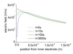
Figure 8: electric field for different times for a cylindrical geometry. Applied voltage=60kV, T=25 ℃.
