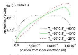
Figure 10: electric field profiles for different temperature gradients after one hour of polarization.
