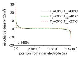
Figure 9: space charge profiles for different temperature gradients after one hour of polarization.
