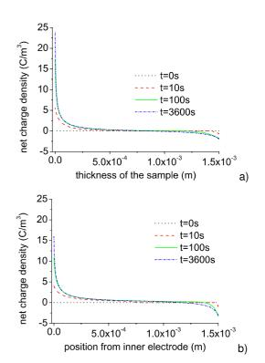
Figure 4: Net charge density function of the distance from electrode for a) a planar geometry, and b) for a cylindrical geometry. Applied voltage=60kV, T=60  $^{\circ}$ C.
