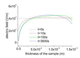
Figure 5: Electric field for different simulation time for a planar geometry. Applied voltage=60kV, T=60 ℃.
