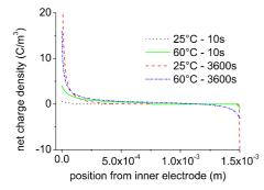
Figure 7: Comparison of the simulated space charge profiles for a cylindrical geometry at 25 °C and at 60 °C.
