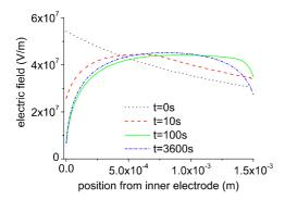
Figure 6: Electric field for different simulation time for a cylindrical geometry. Applied voltage=60kV, T=60 °C.
