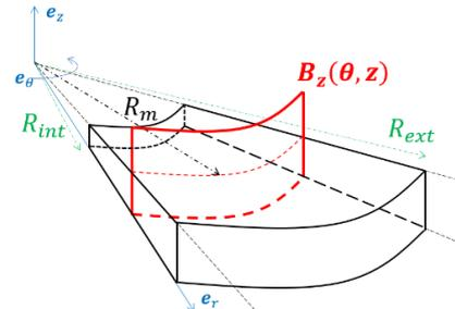
Fig. 4. 2D surface (in red) used to model the AFPM motor.
