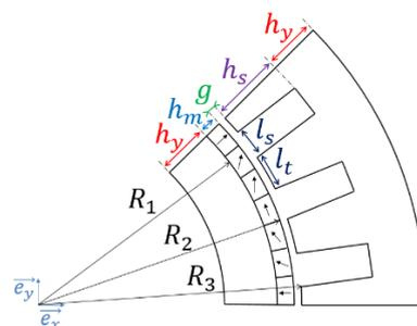
Fig. 1. Geometrical parameters of the RFPM motors [15].
