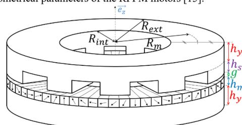
Fig. 2. Geometrical parameters of the AFPM motors.
