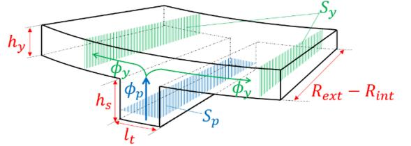
Fig. 7. Flux paths in the AFPM machine.
