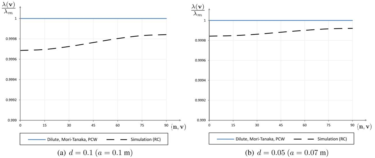
**Fig. 8.** Generalized thermal conductivity  $\lambda(\mathbf{v})$  normalized by its initial value for a material weakened by a single array of parallel closed microcracks of unit normal  $\mathbf{n}$  (RC;  $\lambda^* = 50\% \lambda_m$ ).
