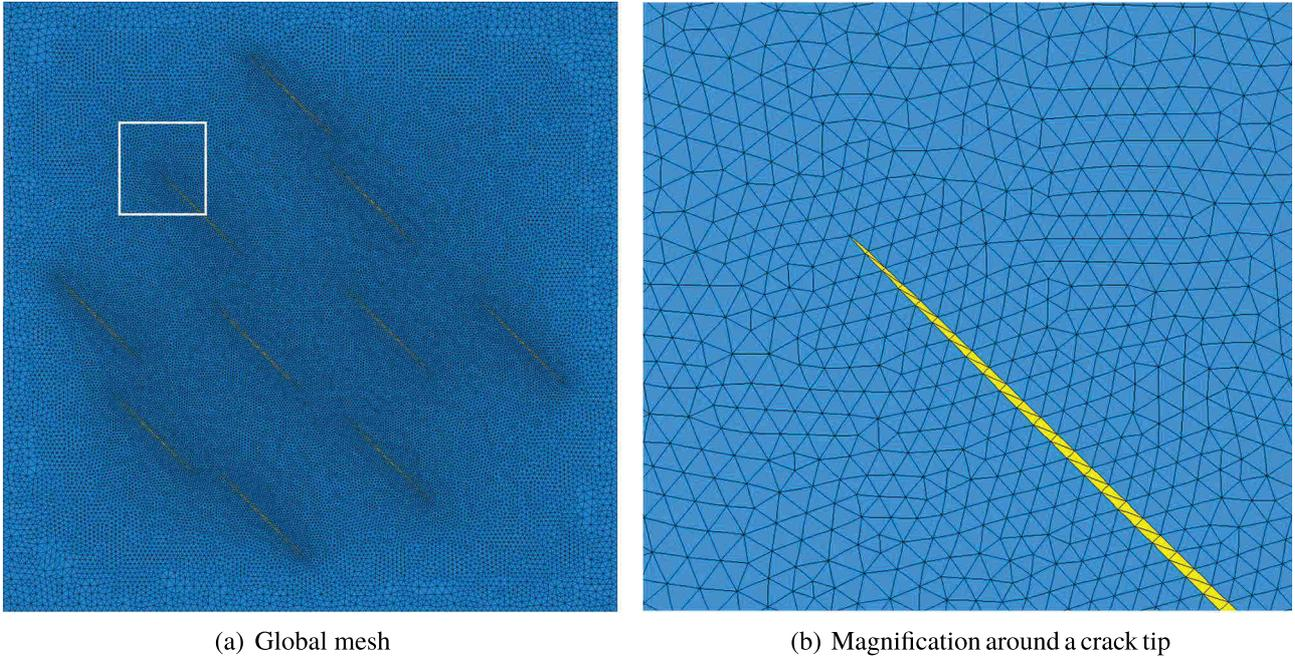
Fig. 3. Simulated area mesh (RC;  $(\mathbf{n}, \mathbf{v}) = 45^\circ$ ).
