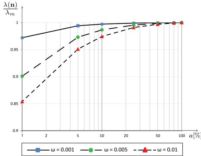
**Fig. 10.** Influence of scalar conductivity  $\lambda^*$  on the normal thermal conductivity  $\lambda(\mathbf{n})$  normalized by its initial value (RC;  $d = 0.1$ ;  $a = 0.1$  m);  $\log_{10}$  scale is used for abscissa.
