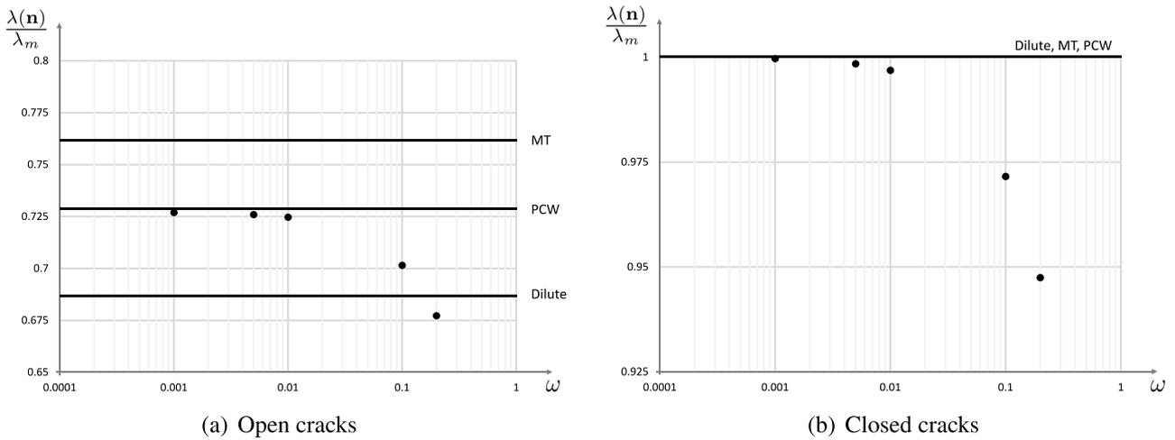
**Fig. 9.** Normal thermal conductivity  $\lambda(\mathbf{n})$  normalized by its initial value for various aspect ratios ( $d = 0.1; a = 0.1$  m); points represent simulation results (RC);  $\log_{10}$  scale is used for abscissa.
