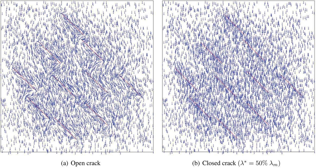
**Fig. 5.** Heat flux vectors at integration points inside the simulated area (RC;  $(\mathbf{n}, \mathbf{v}) = 45^\circ$ ;  $d = 0.1$ ;  $a = 0.1$  m;  $\omega = 0.001$ ).
