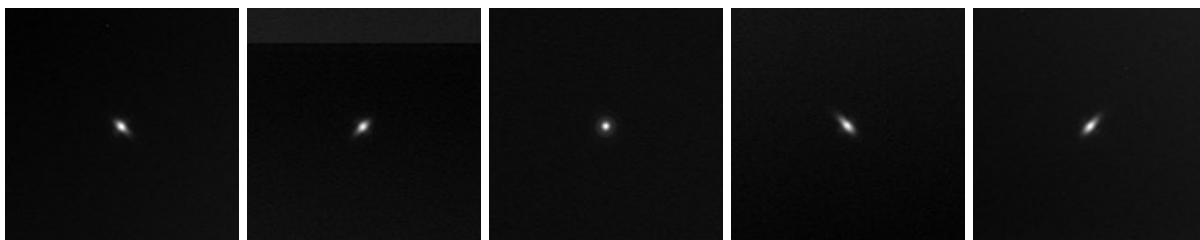
Figure 7. Set of 5 images (center + corners) after coarse alignment but before fine alignment of the final testbed version using the custom aspheric optics. The on-axis central PSF is diffraction limited, but the corners of the field of view show radially elongated PSFs due to z axis misalignment of the powered optics. Completion of the fine optical alignment to achieve diffraction limited PSF quality over the entire field of view is expected in the immediate future as of this writing.
