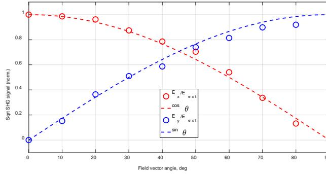
Fig. 4 Horizontal ( $x$ ) and vertical ( $y$ ) components of the peak-normalized, square-rooted E-FISH signals as a function of the field vector angle,  $\theta$ . For a given angle  $\theta$ , the horizontal and vertical components of an applied field  $E_{ext}$  vary as  $E_{ext} \cos \theta$  and  $E_{ext} \sin \theta$ , respectively.
