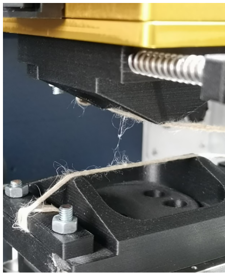
Fig. 8. Entanglement of surface fibers observed after the friction test of flax plain tows. (For interpretation of the references to colour in this figure legend, the reader is referred to the web version of this article.)
