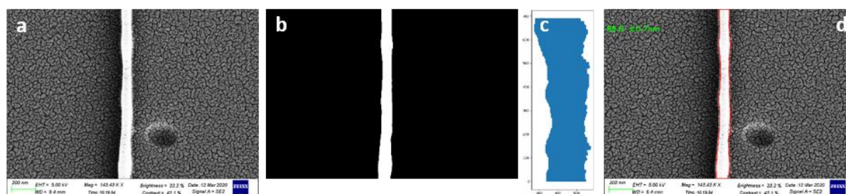
Figure S22. Description of the different steps of the Python script: a) the original image; b) the same image after thresholding; c) the plot of white pixel coordinates; d) the detected contour is shown in red and the average width and the associated error is indicated in green on the final picture.
