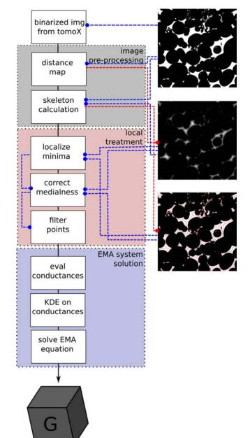
Fig. 5 Graphical representation of the proposed image-based EMA algorithm for permeability estimation directly from 3D binary images
