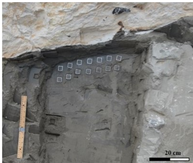
Figure 5. Aluminum sample boxes pushed into the glaciolacustrine mud at Møns Klint, immediately underlying the Upper Cretaceous chalk that has been thrust over it from left to right. After excavation of the boxes, the mud was transferred to plastic boxes for storage, sealing, and subsequent AMS analysis.
