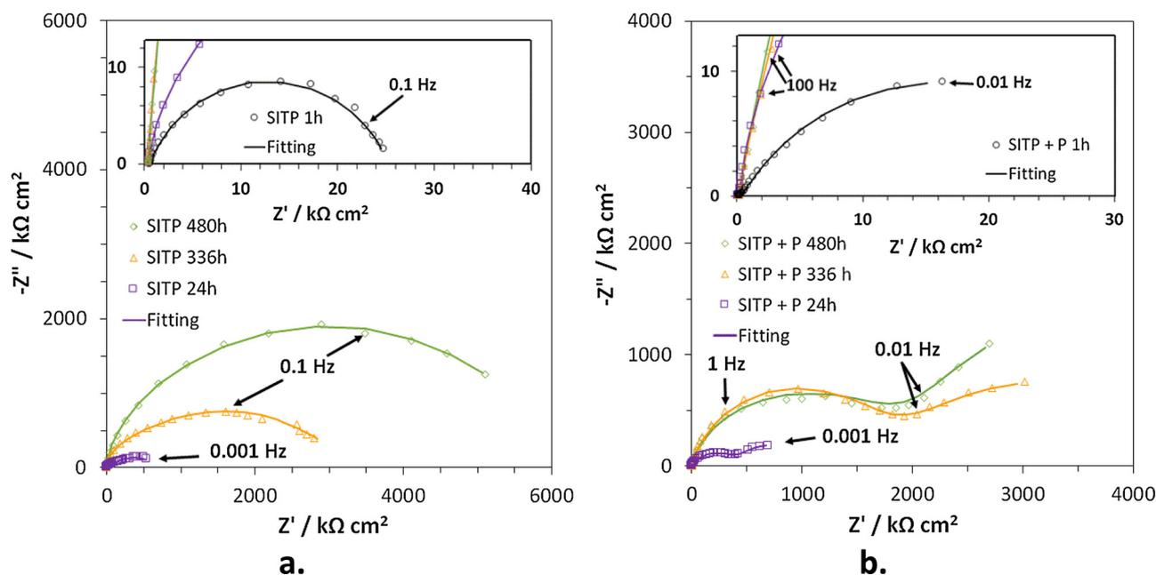
Fig. 8. Nyquist diagrams from EIS tests carried out on bronze immersed for different times in ARX10 solution in the presence of SITS (a) and SITS + P (b). The insets show the complete spectra obtained after 1 h in the presence of SITS (a) and SITS + P (b).
