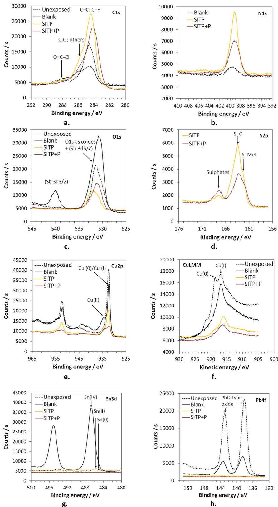
**Fig. 13.** XPS core level spectra of C1s (a), N1s (b), O1s (c), S2p (d), Cu Auger LMM (e), Cu2p (f), Sn3d (g) and Pb4f (h), collected on the unexposed sample and on samples exposed for 480 h to uninhibited (Blank) or inhibited (SITP or SITP + P) ARX10 solution.
