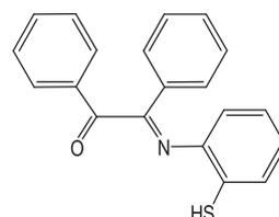
Fig. 1. Structural formulas of the Schiff bases studied as bronze corrosion inhibitors.
