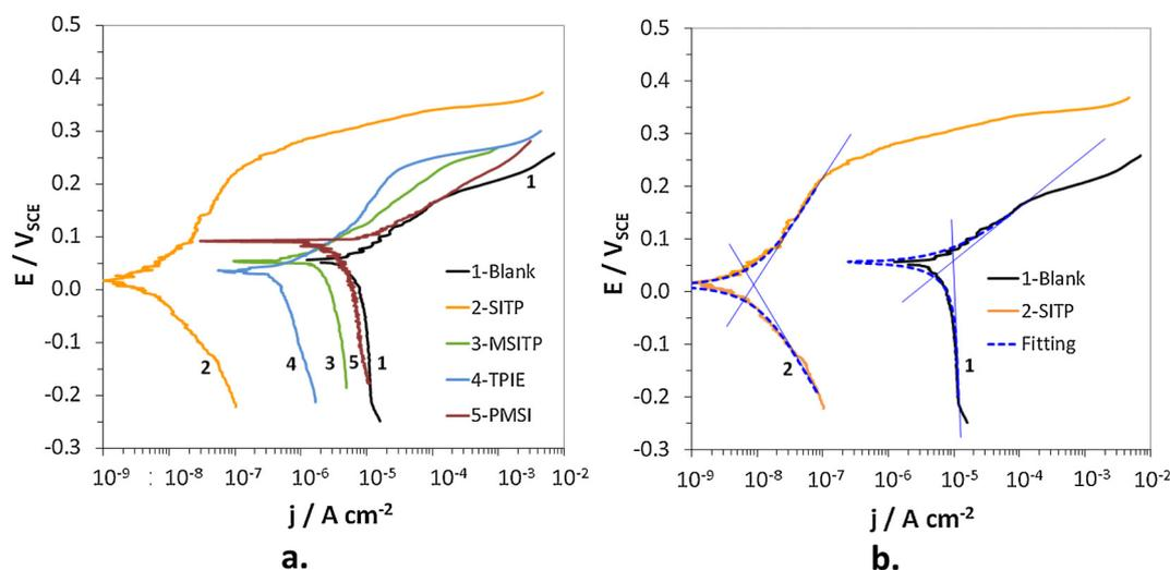
**Fig. 3.** Polarization curves recorded on bronze after 480 h of immersion in ARX10 solution: a) in the absence (1) and in the presence of SITP (2), MSITP (3), TPIE (4) and PMSI (5); b) comparison of experimental and calculated  $E/j$  curves to evaluate the corrosion current density,  $j_{cor}$ .
