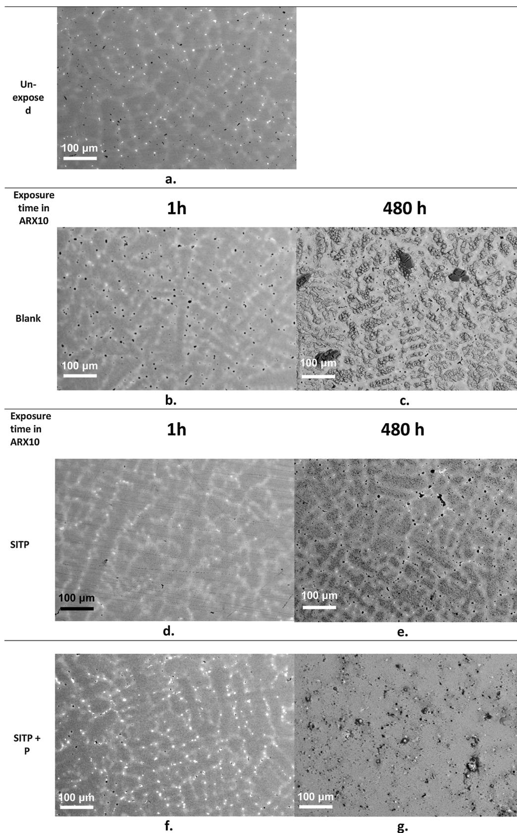
Fig. 11. BSE-SEM micrographs obtained on bare bronze samples (a) and on samples after 1 h (b,d,f) or 480 h (c,e,g) of immersion in ARX10 solution, both in the absence of inhibitors and in the presence of SITP or SITP + P.
