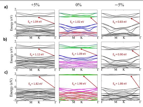
**Figure 3.** Band structures taking into account SOC for (a)  $Cl_3-Cr_2-I_3$ , (b)  $Br_3-Cr_2-I_3$ , and (c)  $Cl_3-Cr_2-Br_3$ , where +5%, 0%, and -5% strain is applied. The red, green, blue, and magenta colors represent the weights of the Cl, Cr, I, and Br atoms, respectively. Red arrows represent the indirect band gap.
