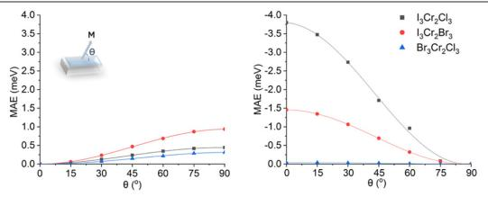
**Figure 6.** Variations of the MAE (per formula unit) with  $\theta$  at (a) +5% strain and (b) -5% strain. The lines are obtained by fitting the data as  $A\sin^2\theta$ .
