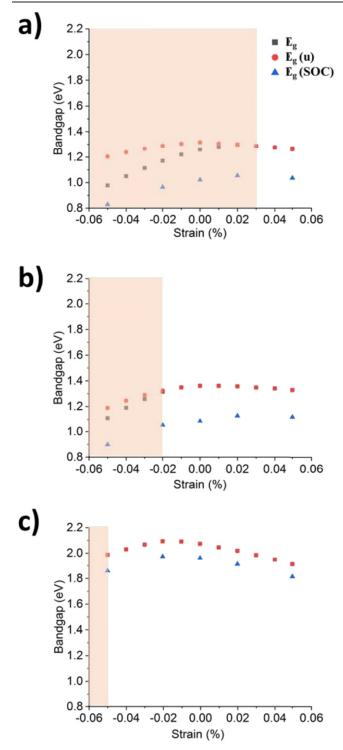
**Figure 4.** Variations of the bandgap  $E_g$  without SOC, bandgap  $E_g$  (u) of the spin up channel without SOC, and bandgap  $E_g(SOC)$  with SOC under strain for (a)  $Cl_3-Cr_2-I_3$ , (b)  $Br_3-Cr_2-I_3$ , and (c)  $Cl_3-Cr_2-Br_3$ . In the highlighted region the easy axis is in-plane.
