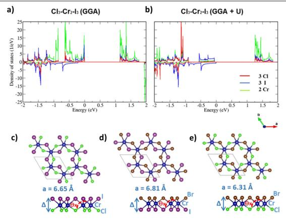
**Figure 1.** (a,b) Effect of the U parameter on the site-projected spin-polarized DOS of  $Cl_3-Cr_2-I_3$ . Top and side views of (c)  $Cl_3-Cr_2-I_3$ , (d)  $Br_3-Cr_2-I_3$ , and (e)  $Cl_3-Cr_2-Br_3$  Janus monolayers.
