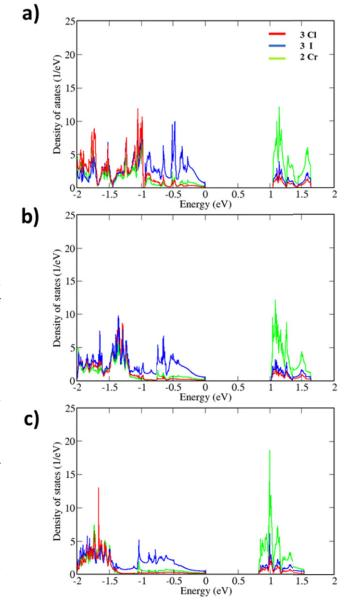
**Figure 5.** Site-projected DOS with SOC under strains of (a) +5%, (b) 0%, and (c) -5% for  $Cl_3-Cr_2-I_3$ .
