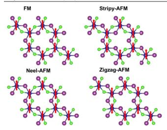
Figure 7. Magnetic orderings considered in the calculations.
