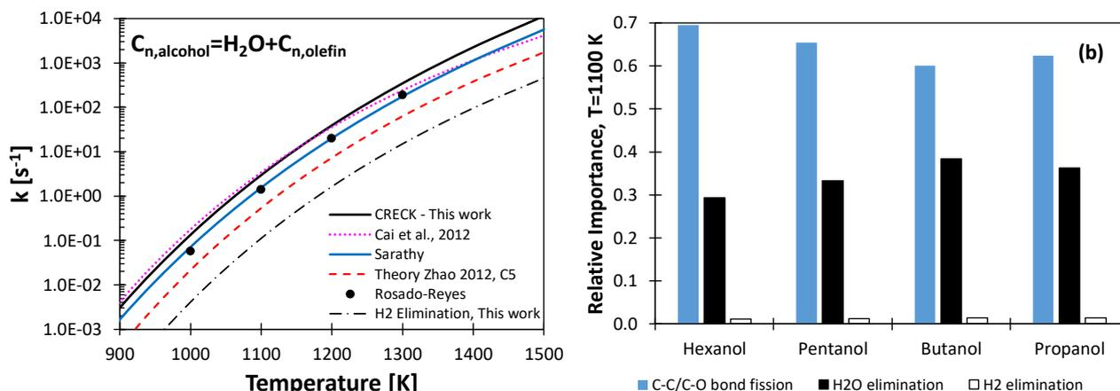
Figure 6. (a) Comparison between rate constants for four-centered molecular dehydration reaction from different sources.<sup>5,78,82,83</sup> (b) Relative contribution of four centered molecular reactions to the total unimolecular decomposition rate of  $n$ -C<sub>3</sub>-C<sub>6</sub> alcohols.
