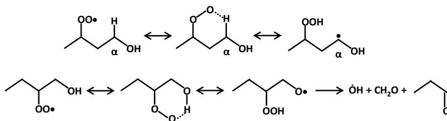
Figure 8. Example 6-membered isomerization reactions in  $n$ -butanol oxidation. The top row shows  $sec\text{-}\dot{R}O_2$  producing  $\alpha\text{-}\dot{Q}OOH$ ; the bottom row shows (Waddington mechanism):  $\beta\text{-}\dot{R}O_2$  producing an hydroperoxy alkoxyradical and its successive decomposition.
