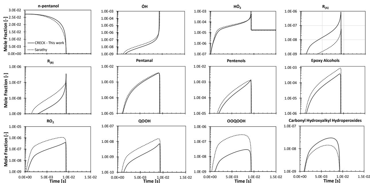
Figure 15. Simulated mole fraction profiles of relevant species in the oxidation of an *n*-pentanol/air mixture in an adiabatic constant volume batch reactor ( $T = 900$  K,  $p = 10$  bar,  $\varphi = 1.0$ ). Solid lines represent the lumped model from this work, dashed lines represent the detailed model from Sarathy et al.<sup>5</sup>
