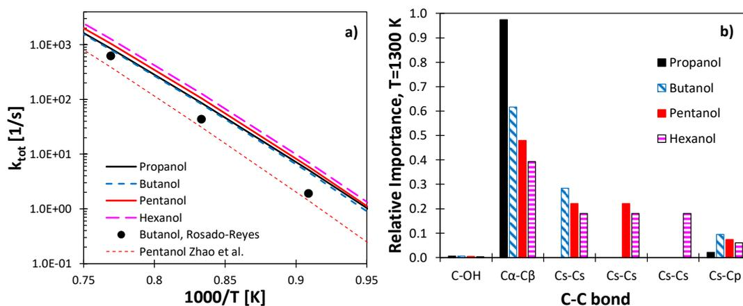
Figure 5. (a) Total decomposition rate constant for *n*- $C_3$ – $C_6$  alcohols obtained from the rate constant values adopted in this work, compared with literature values.<sup>78,82</sup> (b) Relative importance of the different unimolecular decomposition channels.
