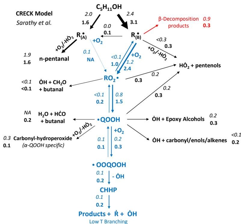
Figure 16. Flux analysis of *n*-pentanol oxidation in an adiabatic constant volume batch reactor at  $T = 900$  K,  $p = 10$  bar, and  $\phi = 1.0$  (fuel conversion of  $\sim 20\%$ ). Numbers are rates of production/consumption in  $10^{-4}$  mol  $cm^{-3}$   $s^{-1}$ . Bold font denotes data obtained using the CRECK model; italic font denotes data obtained from Sarathy et al.<sup>5</sup> NA indicates that the pathway was not available in the model.
