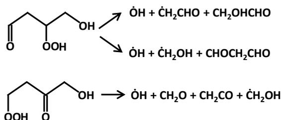
Figure 12. Example of CHHP branching decomposition reactions.
