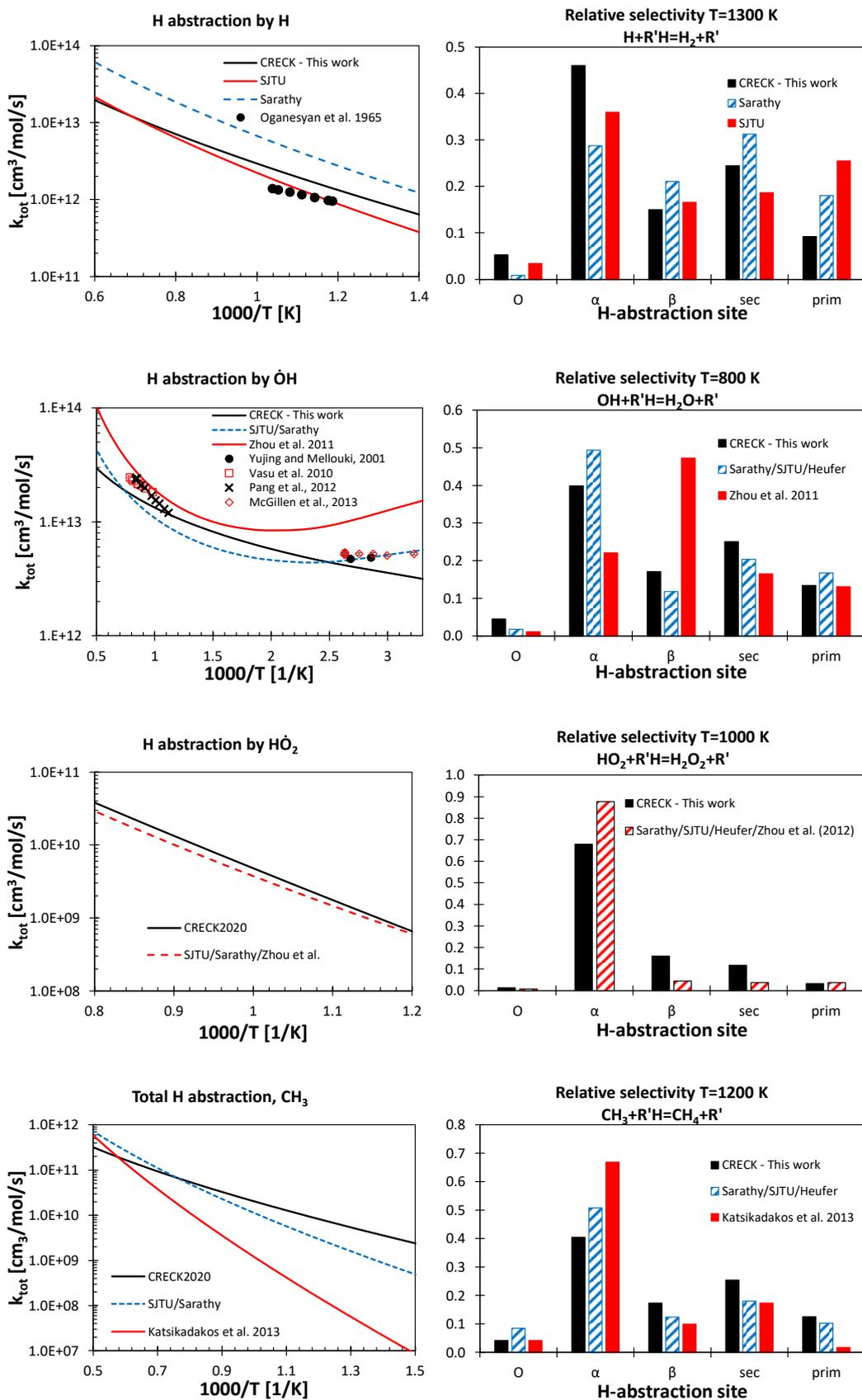
Figure 7. (Left) Total rate constants of H-atom abstraction reactions by  $\dot{\text{H}}$ ,  $\dot{\text{OH}}$ ,  $\dot{\text{HO}}_2$ , and  $\dot{\text{C}}\text{H}_3$  on *n*-butanol from this work (black) and from the literature.<sup>5,41–45,48,49,83,87</sup> (Right) Relative selectivity to the different H-atom abstraction site for *n*-butanol from this work (black) and from the literature.
