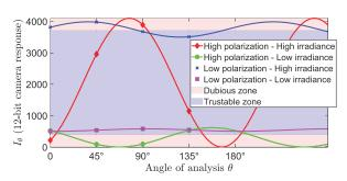
**Fig. 2.** Simulated theoretical polarization camera responses, with a varying input signal according to the Malus law.
