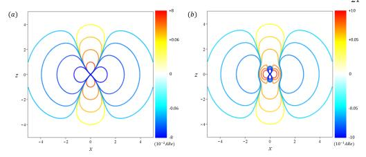
FIGURE 5. Contours of the y-averaged pressure  $\langle \tilde{p} \rangle$ : (a)  $\gamma = 0$  and (b)  $\gamma = 15$ , cf. Eq. (4.5).
