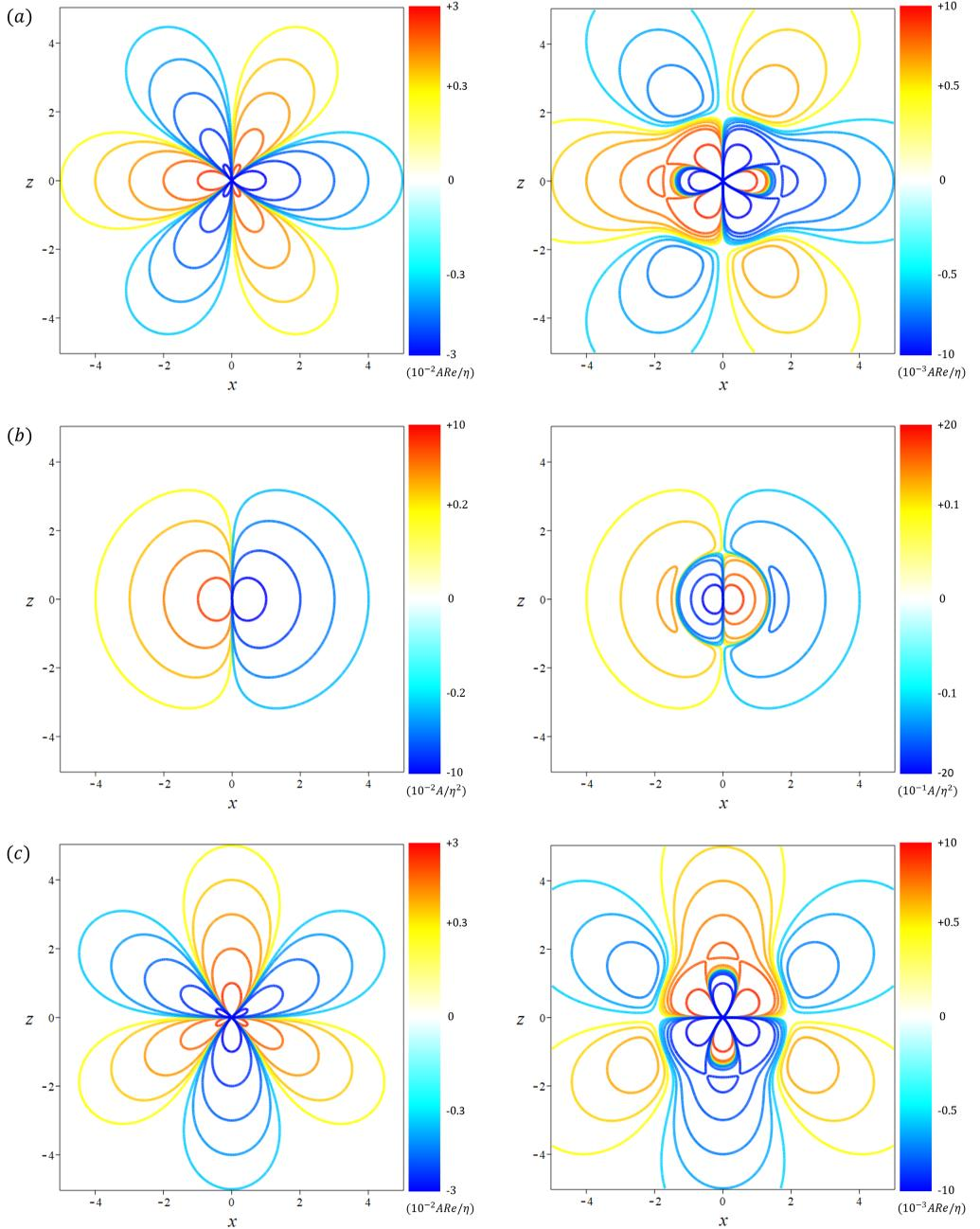
FIGURE 3. Contour plots for the  $y$ -averaged (a) streamwise velocity  $\langle \tilde{u}_x \rangle$ , cf. Eq. (4.1); (b) wall-normal velocity  $\langle \tilde{u}_y \rangle$ , cf. Eq. (4.3) and; (c) spanwise velocity  $\langle \tilde{u}_z \rangle$ , cf. Eq. (4.2). The left and right columns correspond to the cases of  $\gamma = 0$  and  $\gamma = 15$ , respectively.
