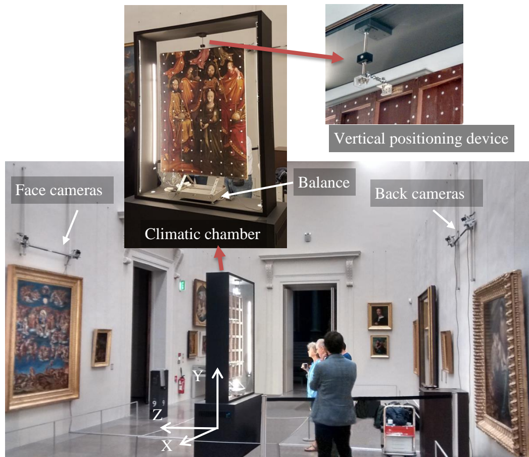
Figure 2 : The apparatus in the museum: climate chamber, optical device and vertical positioning device
