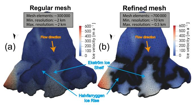
**Figure 4.** The 3-D plot of the model domain showing the two main mesh resolutions employed in this study. (a) shows uniform mesh of 2 km resolution and (b) shows refined mesh in areas of interest such as the grounding line and the ice-rise divides. In these areas the mesh resolution is  $\sim 500$  m and away from these regions the mesh resolution increases to 10 km.
