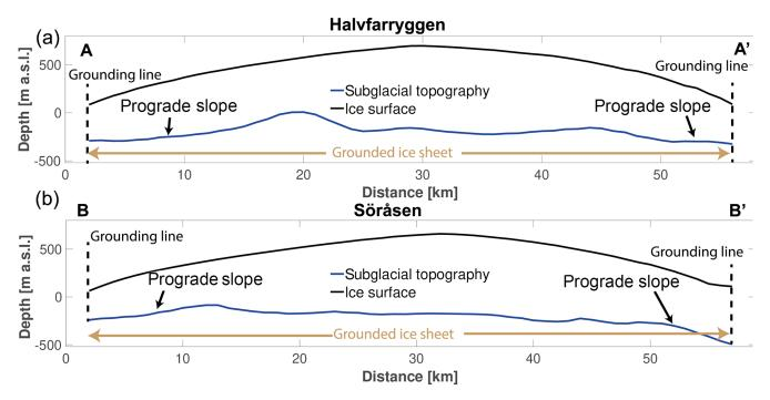
**Figure 12.** Cross sections of grounded subglacial topography from the BEDMAP2 dataset (Fretwell et al., 2013) for the **(a)** Halvfarryggen and **(b)** Söråsen ice rises, underlining the prograde sloping subglacial topography of both ice rises in the vicinity of the current grounding line.
