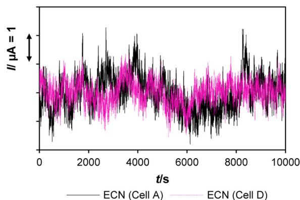
**Fig. 10.** Variations of typical current noise ( $I/\text{nA} = f(t)$ ) obtained in flow cell A (inoculation with *Desulfovibrio alaskensis*) and flow cell D (inoculation with *Desulfovibrio desulfuricans*) recorded 12 h after first antimicrobial treatment ( $t_e = 1087$  h). Data linearly detrended.
