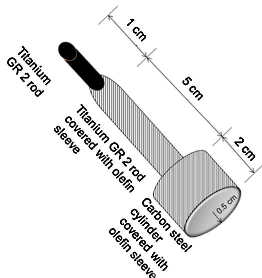
Fig. 3. Working electrode scheme.
