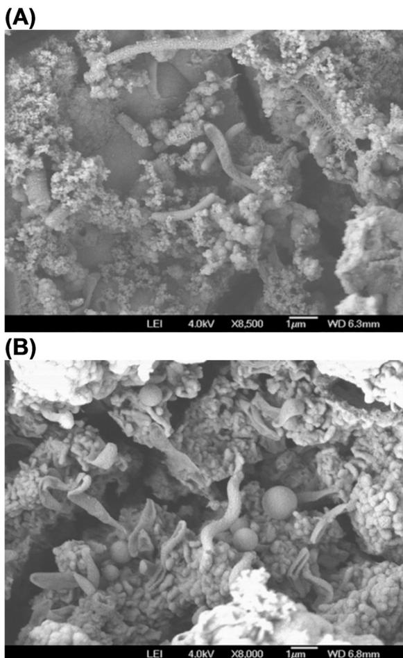
**Fig. 8.** SEM of steel specimens placed at 6 o'clock position and retrieved from flow cells after 1070 h of exposure: (A) specimen from cell A (inoculation with *Desulfovibrio alaskensis*)—8500 $\times$ ; (B) specimen from cell D (inoculation with *Desulfovibrio desulfuricans*)—8000 $\times$ .
