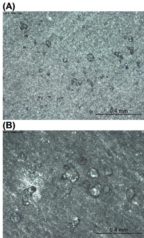
**Fig. 9.** Micro photographs (100 $\times$ ) of steel specimens retrieved from flow cells after 1070 h of exposure and after corrosion product removal, revealing localized corrosion attacks: (A) specimen from flow cell A (inoculation with *Desulfovibrio alaskensis*); (B) specimen from flow cell D (inoculation with *Desulfovibrio desulfuricans*).
