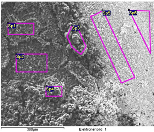
**Fig. 14.** SEM micrograph (100 $\times$ ) with emphasized areas submitted to EDX analysis of 12 o'clock positioned specimen exposed in flow cell A (inoculation with *Desulfovibrio alaskensis*) for 2200 h.
