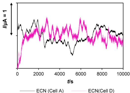
**Fig. 12.** Variations of typical current noise ( $I/nA=f(t)$ ) obtained in flow cell A (inoculation with *Desulfovibrio alaskensis*) and flow cell D (inoculation with *Desulfovibrio desulfuricans*) recorded 12 h after the second antimicrobial treatment ( $t_e = 2192$  h). Data linearly detrended.
