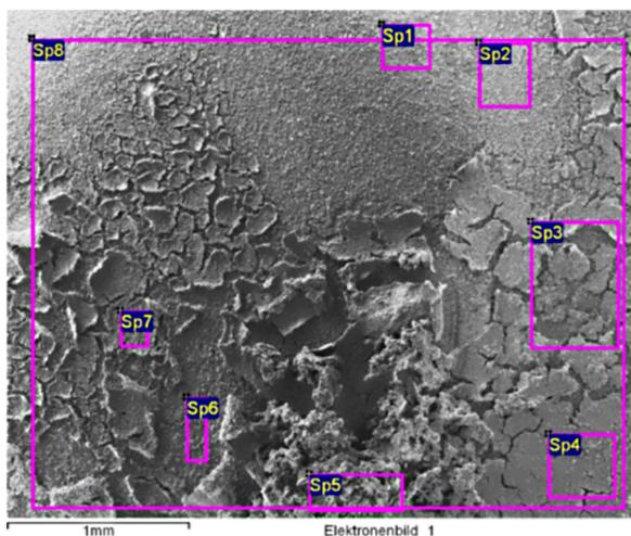
**Fig. 16.** SEM micrograph (100 $\times$ ) with emphasized areas submitted to EDX analysis of 12 o'clock positioned specimen exposed in flow cell D (inoculation with *Desulfovibrio desulfuricans*) for 2200 h.
