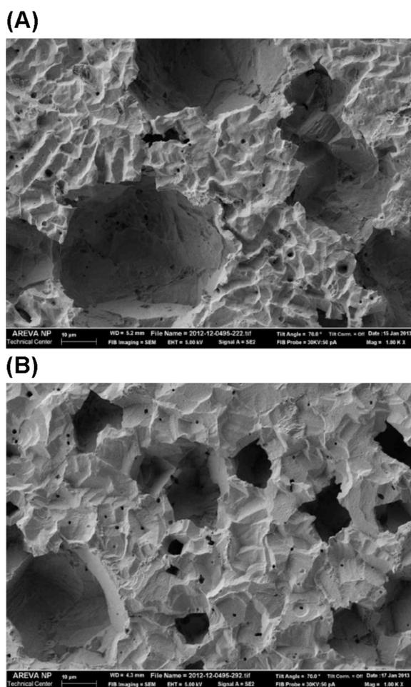
**Fig. 18.** SEM micrographs (1000 $\times$ ) of 12 o'clock positioned steel specimens retrieved after 2200 of immersion in flow cells and chemically cleaned from corrosion deposits: (A) specimen from flow cell A (inoculation with *Desulfovibrio alaskensis*); (B) specimen from flow cell D (inoculation with *Desulfovibrio desulfuricans*).
