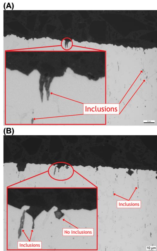
**Fig. 22.** Cross-sections micrographs of 12 o'clock positioned specimen exposed in cell D (inoculation with *Desulfovibrio desulfuricans*) for 2200 h after corrosion product removal: (A) Micrograph showing beginning of corrosion attack on location of MnS inclusion; (B) Micrograph showing beginning of corrosion attack in presence and absence of MnS inclusion.
