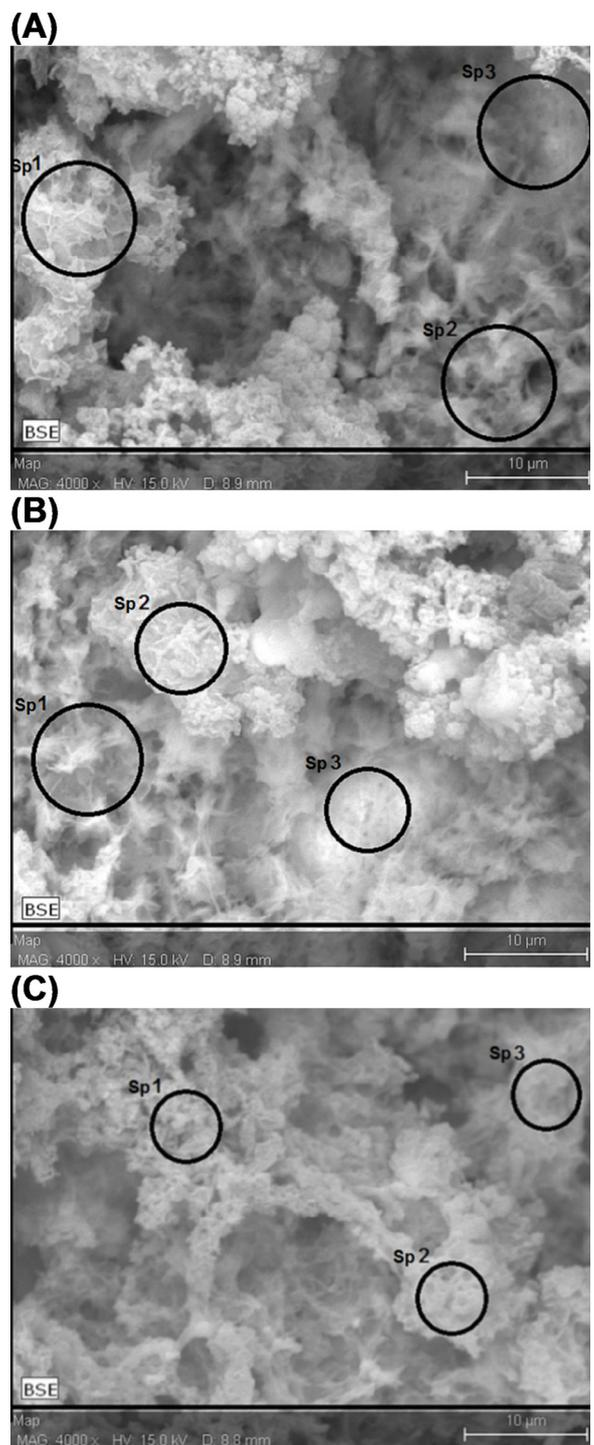
**Fig. 13.** SEM micrographs ( $4000\times$ ) with emphasized areas submitted to EDX analysis of four 6 o'clock positioned specimens exposed in flow cell A (inoculation with *Desulfovibrio alaskensis*) for 2200 h.
