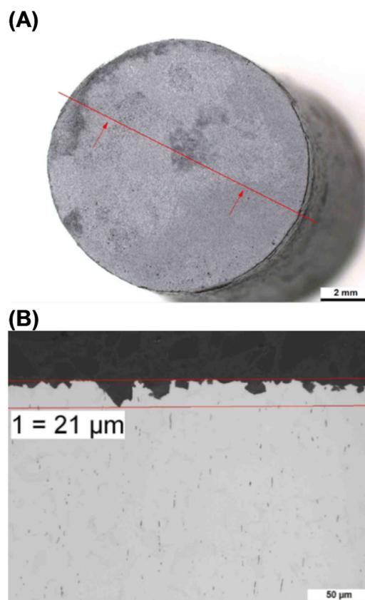
**Fig. 20.** Macrograph and micrograph of 12 o'clock positioned specimen exposed in cell D (inoculation with *Desulfovibrio desulfuricans*) for 2200 h after corrosion product removal: (A) Macrograph before cross section and cutting line; (B) Micrograph for depth determination of attack.
