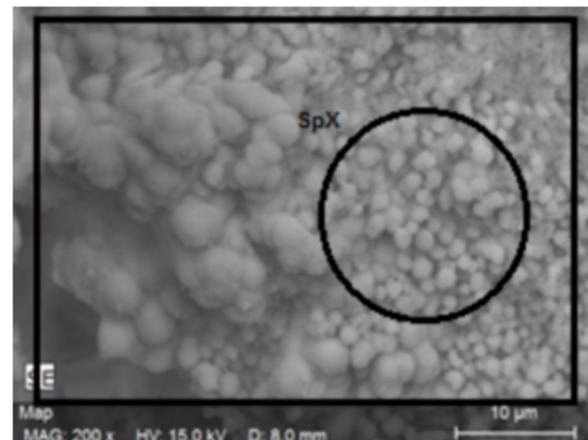
**Fig. 15.** SEM micrographs (4000 $\times$ ) with emphasized areas submitted to EDX analysis of three 6 o'clock positioned specimens exposed in cell D (inoculation with *Desulfovibrio desulfuricans*) for 2200 h.
