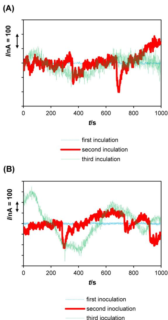
**Fig. 7.** Variations of typical current noise ( $I/nA=f(t)$ ) obtained during the second test stage ( $t_e=792-1070$  h) obtained 24 h after each inoculation: (A) in flow cell D (inoculation with *Desulfovibrio desulfuricans*); (B) in flow cell A (inoculation with *Desulfovibrio alaskensis*). Data linearly detrended.
