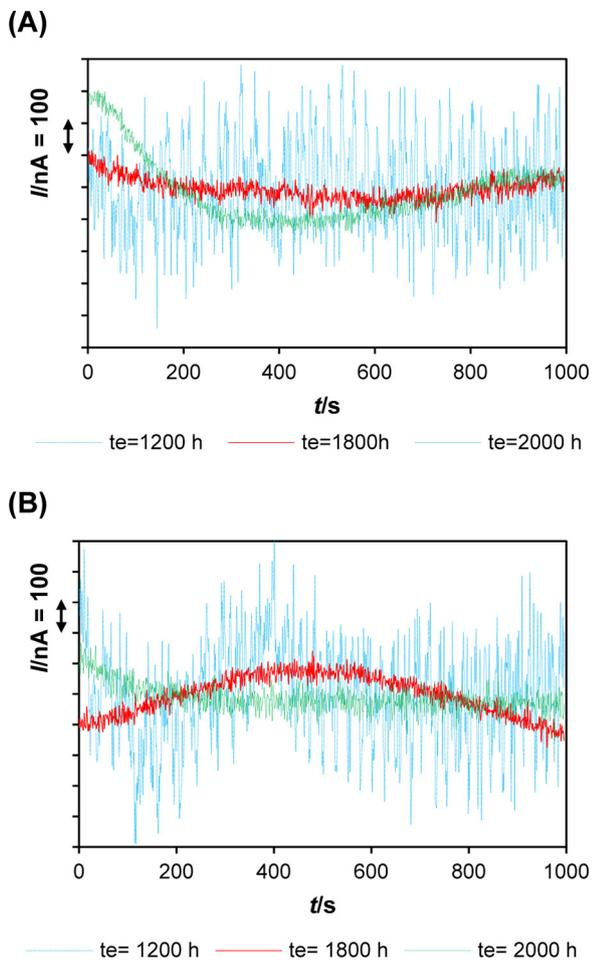
**Fig. 11.** Variations of typical current noise ( $I/nA=f(t)$ ) obtained during the third test stage ( $t_e = 1070\text{--}2200$  h) at  $t_e = 1200$  h,  $t_e = 1800$  h and  $t_e = 2180$  h: (A) in flow cell D (inoculation with *Desulfovibrio desulfuricans*); (B) in flow cell A (inoculation with *Desulfovibrio alaskensis*). Data linearly detrended.
