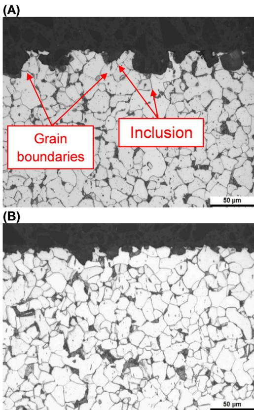
**Fig. 21.** Etched cross-sections SEM micrographs (250 $\times$ ) of 12 o'clock positioned specimen exposed for 2200 h: (A) from flow cell A (inoculation with *Desulfovibrio alaskensis*); (B) from flow cell D (inoculation with *Desulfovibrio desulfuricans*).
