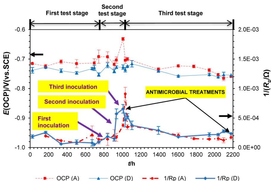
**Fig. 5.** Average instantaneous corrosion rate ( $1/(R_p/\Omega)$ ) and OCP ( $E(OCP)/V$  vs. SCE) values with standard deviation error bars for 12 o'clock positioned steel specimens (WE) exposed in flow cell A (inoculation with *Desulfovibrio alaskensis*) and flow cell D (inoculation with *Desulfovibrio desulfuricans*) during the 2200 h of test.
