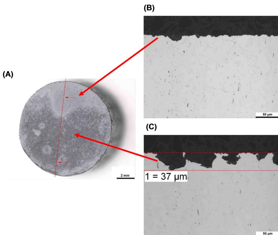
**Fig. 19.** Macrographs and micrographs of 12 o'clock positioned specimen exposed in cell A (inoculation with *Desulfovibrio alaskensis*) for 2200 h after corrosion product removal: (A) Macrograph before cross section and cutting line; (B) Micrograph for depth determination of attack in more lighted coloured region; (C) Micrograph for depth determination of attack in darker coloured region.
