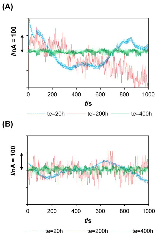
**Fig. 6.** Variations of typical current noise ( $I/nA=f(t)$ ) obtained during the first test stage ( $t_e=0-792$  h, prior to inoculations) at  $t_e=20$  h,  $t_e=200$  h and  $t_e=400$  h: (A) in flow cell D (inoculation with *Desulfovibrio desulfuricans*); (B) in flow cell A (inoculation with *Desulfovibrio alaskensis*). Data linearly detrended.
