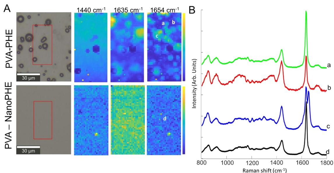
Figure 4: A: White light images of the PVA PHE and PVA-NanoPHE films with corresponding intensity maps at 1440 cm<sup>-1</sup>, 1635 cm<sup>-1</sup> and 1654 cm<sup>-1</sup>. B: Raman spectra extracted from position labelled a, b, c and d on images. Spectra offset for clarity.
