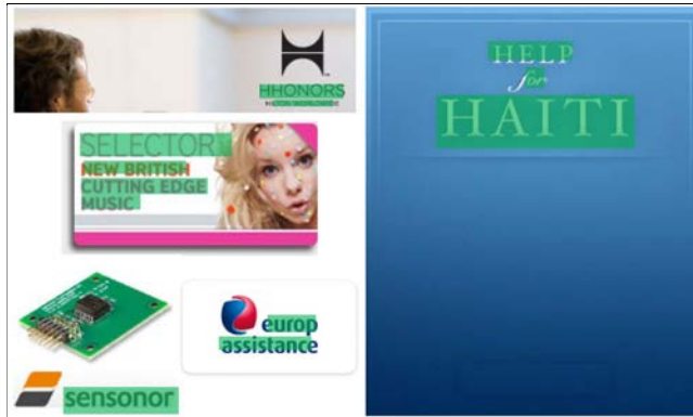
Fig. 5. Example text detection results of the proposed method. The images are 5 test images of different resolutions from the born-digital images dataset in [16]. The detection results are shown in green boxes. The green regions are in most of the cases accurate and cover words or textlines of the text.
