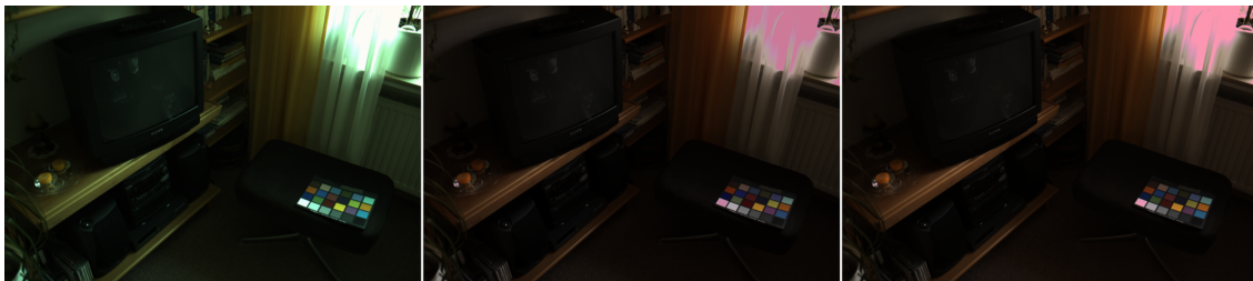
Figure 7: Left: original image. Middle: Yilmaz correction. Right: diagonal correction. The illuminant estimation in both corrections was done using the white square present on the color checker.
