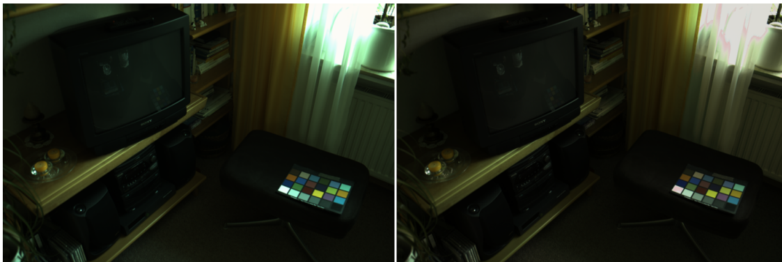
Figure 8: Left: original image. Right: Yilmaz correction. The pixels that were supposed to be clipped after the correction have been left unchanged from the original image.
