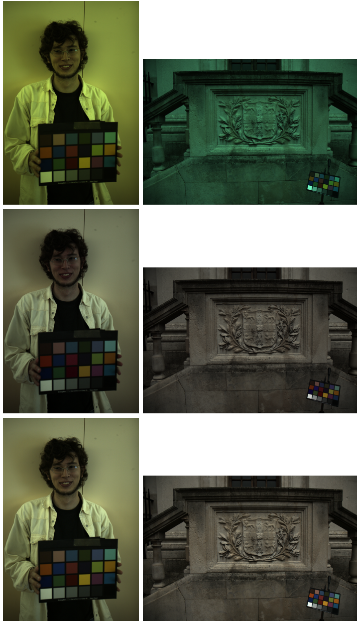
Figure 2: Top: original images from ColorChecker dataset. Middle: result of Yilmaz’s ACC algorithm. Bottom: diagonal correction.
