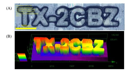
Figure 13 Optical microscopy of the three-dimensional pattern obtained from TX-2CBZ/Iod/EDB (0.07/2.0/2.0 w/w/wt%) in a TMPTA/EPOX blend (50/50 w/wt%) (A) 2D panorama, (B) 3D panorama
