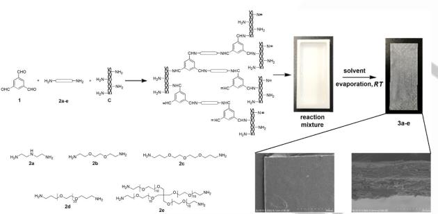
Scheme 1. Synthesis and preparation of the dynameric collagen membranes 3 a-e from collagen, C and dynameric frameworks of trialdehyde core centers 1 and polyamine connectors 2 a-e. Surface (3 e) and cross-section (3 a) images of the membranes have been obtained via scanning electronic microscoppy (SEM).
