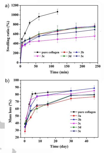
Figure 2. a) Swelling kinetics and b) degradation profile of the collagen, C and dynameric collagen **3 a**-**e** membranes from PBS (pH 7.4) at 37 °C.
