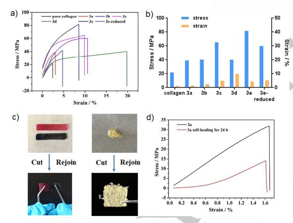
Figure 1. a) Tensile stress-strain curves collagen C, dynameric collagen 3a-e membranes and reduced 3e membrane. b) The highest tensile stress and break strain for each membrane. c) Cutting and rejoining of the self-healing membranes. d) Stress-strain curves of the original and the re-healed membrane 3a.
