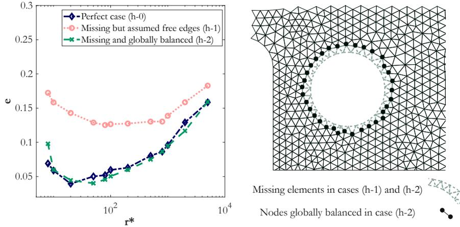
Figure 8: Influence of preprocessing choice for the hole edge definition on the error as a function of  $r^*$  for a given  $C$ , for the cases of an imperfectly defined edge close to the hole (with (h-1) the assumption of free edge, (h-2) the global balance condition) and of a perfectly defined edge (h-0) (left subfigure). Nodes/elements used in the calculations (right subfigure).
