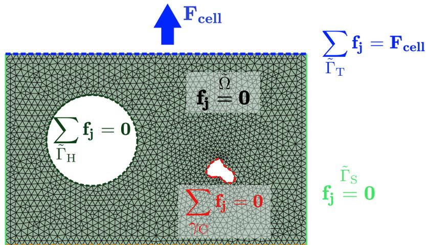
Figure 11: Summary of the proper preprocessing choice to deal with three particular boundaries (top boundary with a global force information, *cluster* of missing data and imperfectly defined edges close to a hole).
