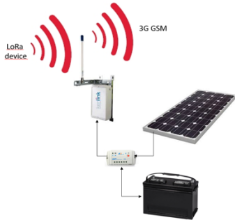
Figure 10: autonomous LoRa antenna system
