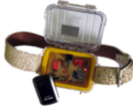
Figure 1 : LynxNet collar device [4]
