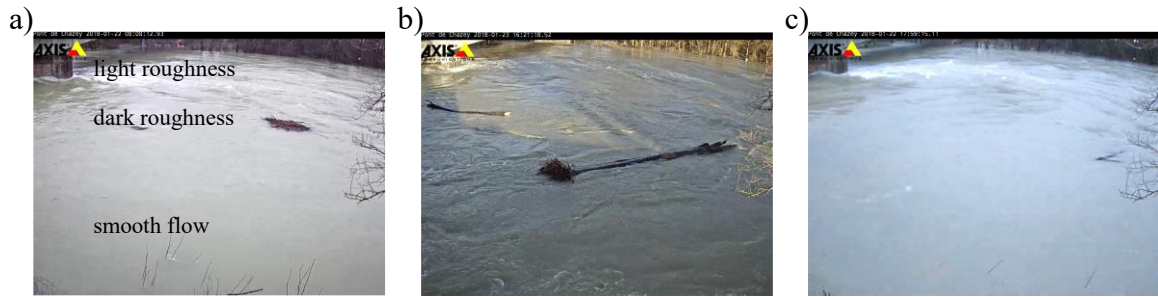
Fig 12 Different light conditions during (a) morning, (b) noon and (c) late afternoon, results in different frame roughness's and different detection performances.
