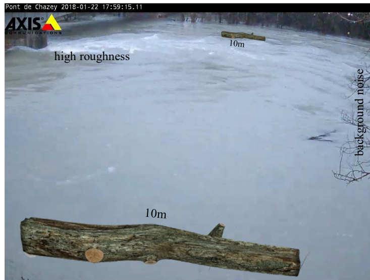
Fig 13 Wood position can highly affect the quality of detection. Pieces that are passing in front of the camera are detected much better than the pieces far from the camera.
