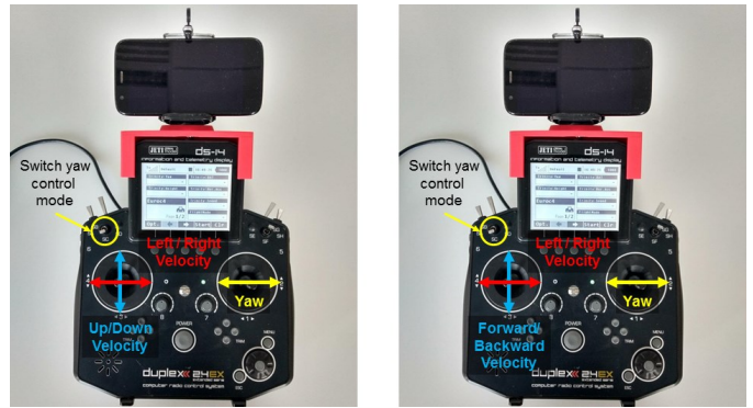
Fig. 6. Tele-operation remote control. Left: sticks configuration for cylinder or vertical planes. Right: sticks configuration for tunnel surface.
