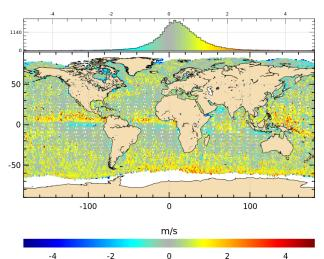
Figure 15: Difference between SWIM nadir altimeter wind and ECMWF wind for SWIM cycle 21 to 28 Map and histogram (on top). Mean=0.32 m/s, Median=0.30 m/s and Standard Deviation=0.92 m/s
