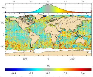
Figure 13 : Difference between SWIM nadir SWH and ECMWF Hs for SWIM cycles 21 to 24: Map and histogram (on top). Mean=0.0362 m, Median=0.0246m, Standard Deviation=0.1478m
