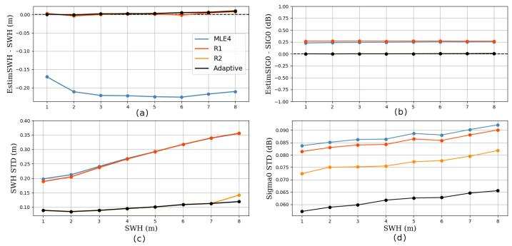
Figure 3 a) SWH biases b)  $\sigma^0$  biases c) SWH standard-deviation d)  $\sigma^0$  standard deviation. Statistics retrieved from MLE4 (blue), R1 (red), R2 (orange) and Adaptive (black) algorithms. Note that in (c), the orange curve for R2 is hidden behind the black one
