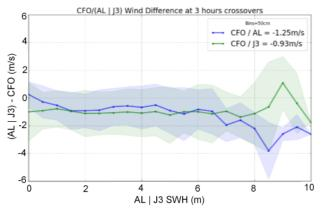
Figure 16 : Bias between SWIM wind and two altimeter missions (SARAL/AltiKa in blue, Jason-3 in green) for SWIM cycle 21 to 28. Each dot of the solid line is the mean computed per box of 50cm of SWH and the envelope represents the associated standard deviation.
