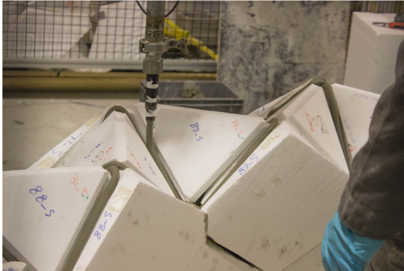
Fig. 8. Free deposition on EPS blocks with correct regime (no coiling, no stretching)
