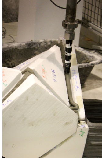
Fig. 5. Coiling pattern (meandering) at the bottom of the gutter.
