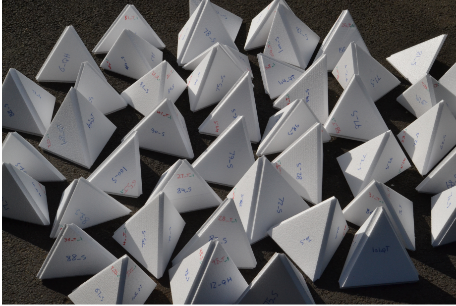
Fig. 7. Robotically hot-wire cut EPS blocks, cut at l’Ecole des Ponts ParisTech (picture: Romain Mesnil)
