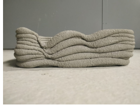
Fig. 4: Longitudinal tearing in the extruded material creating discontinuous layers (photo credits: Paul Carneau)
