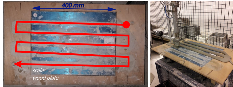
Fig. 7: left : Experimental apparatus with a scale and surrounded plate, and toolpath to measure the force applied during the extrusion, right : On-going printing of the layers on the scale (photo credits: Romain Mesnil).
