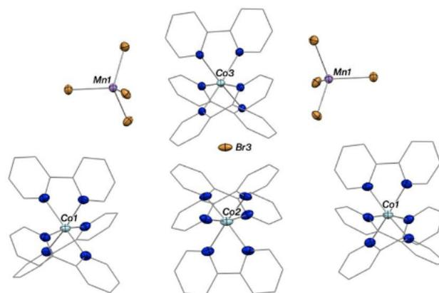
**Figure 1.** ORTEP of reduced cobalt complex **Co-Red** [3 [Co<sup>I</sup>-Bipy<sub>3</sub>]<sup>+</sup>; [Co<sup>II</sup>Bipy<sub>3</sub>]<sup>2+</sup>; 2 [MnBr<sub>4</sub>]<sup>2-</sup>; Br<sup>-</sup>] at 50% probability ellipsoids with H atoms and solvent omitted and 2,2'-bipyridine ligands in wireframe for clarity.
