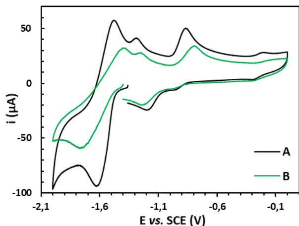
**Figure 2.** Cyclic voltammograms of **A** and **B** in DMF. **A**: 1 mM [Co<sup>I</sup>Bipy<sub>3</sub>]<sup>+</sup>; **B**: 1 mM [Co<sup>I</sup>Bipy<sub>3</sub>]<sup>+</sup> mixed beforehand with **1** in DMF; glassy carbon working electrode; scan rate 1 V.s<sup>-1</sup>. Supporting electrolyte: 100 mM tetrabutylammonium tetrafluoroborate. See SI S.7 for full experiment details.
