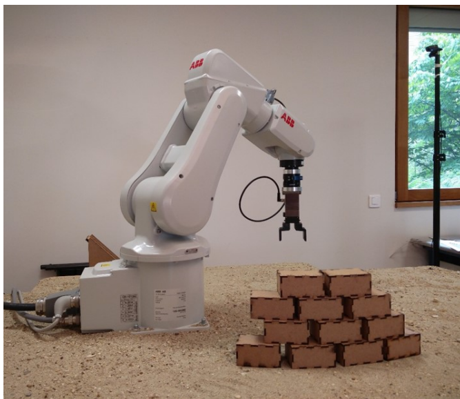
(b) Wall built using artificial vision algorithm for block location and placement estimation
