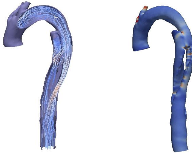
Figure 2: FSI simulation at systolic phase (Left: streamlines colored by velocity magnitude; Right: wall shear stress).
