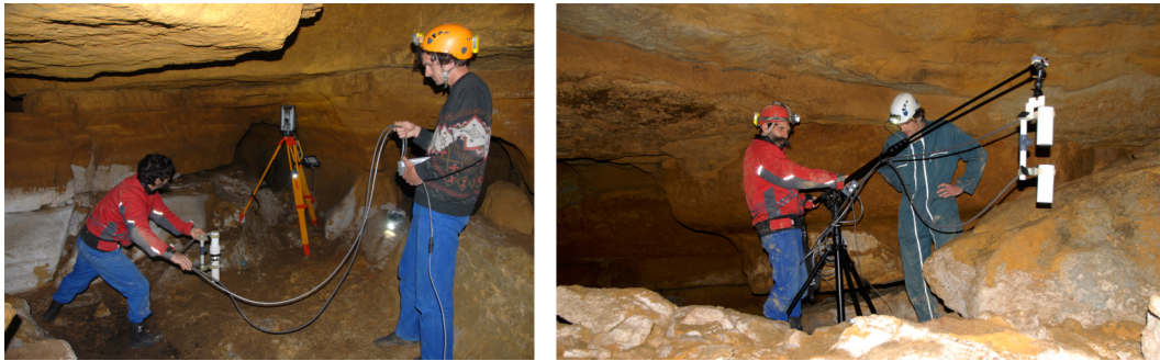
Fig. 6: Protocol of 3D magnetic prospection in the cave of “Les Fraux”.
