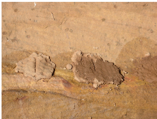
Fig. 2. Mechanical resistance test on soil no. 1, without straw on the left, with straw on the right.
