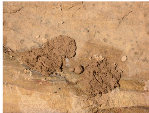
Fig. 3. Mechanical resistance test on soil no. 2, without straw on the left, with straw on the right.
