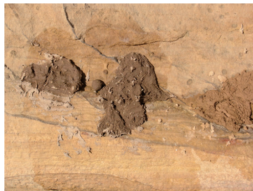
Fig. 4. Mechanical resistance test on soil no. 3, without straw on the left, with straw on the right.
