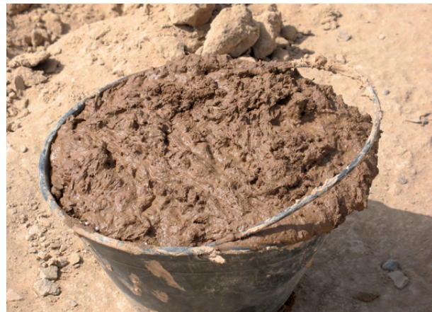
Fig. 20. Mud (for building) ready to use.
