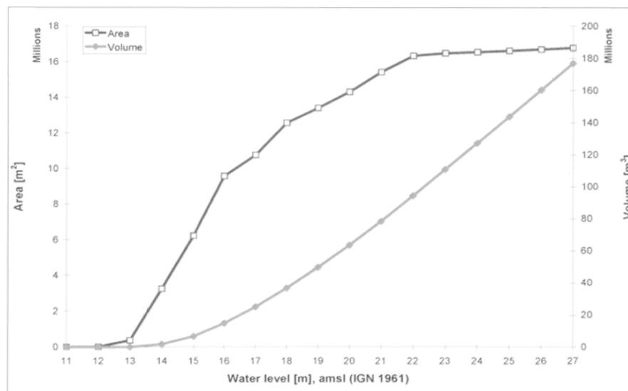
**Fig. 5(b).** Area/volume plot of water in the West Baray, based on a digital elevation model (DEM) that combines the TOPSAR elevation model and bathymetric survey data (IGN/FARK 1961, published in Pottier, 1993; Pl. 2-3). The DEM was used to calculate the volume-to-area water level curve using ArcGIS 8.3, which was then used to convert the water height within the baray (m AMSL) to volume (m<sup>3</sup>).
