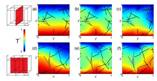
FIG. 7. The temperature field in the two orthogonal vertical midplanes at steady state for three different dimensionless fracture transmissivities: (a), (d)  $\sigma' = 0.1$ ; (b), (e) 1; and (c), (f) 5. Data for  $\rho' = 4$  and  $Ra_m = 41.5$ .
