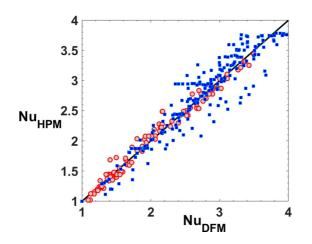
FIG. 12. The Nusselt number  $Nu_{HPM}$  computed in a homogeneous porous medium vs the Nusselt number  $Nu_{FPM}$  computed in the discrete fracture medium, both presenting the same effective permeability. Data for two-dimensional convection (red dots) and three-dimensional convection (blue squares); one dot represents one realization, and the first bisector is shown. Additional data: 7 <  $Ra_m < 139, 0.5 < \rho' < 10$ , and  $0.1 < \sigma' < 10$ .
