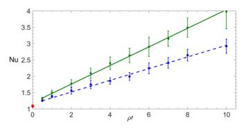
FIG. 10. The average Nusselt number as a function of the dimensionless fracture density  $\rho'$  for  $\sigma' = 1$  (blue circles),  $\sigma' = 2$  (green squares), and  $Ra_m = 41.5$  (the red star represents  $Nu_{mat}$ ). Solid and broken lines are the linear fits [Eqs. (25a) and (25b)].
