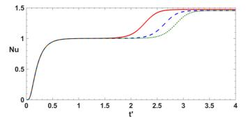
FIG. 3. The Nusselt number as a function of time for Ra = 50 in a square unit box. Data for  $\delta'_M = 0.033$  (solid red line), 0.025 (dashed blue line), and 0.017 (dotted green line).
