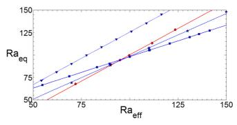
FIG. 16. The equivalent Rayleigh number  $Ra_{eq}$  as a function of the effective Rayleigh number  $Ra_{eff}$  for four individual fracture networks. Data for  $\rho' = 1$ ,  $\sigma' = 5$  (red circles);  $\rho' = 3$ ,  $\sigma' = 5$  (blue triangles);  $\rho' = 4$ ,  $\sigma' = 0.1$  (blue squares); and  $\rho' = 8$ ,  $\sigma' = 1$  (blue stars). Solid and broken lines correspond to Eq. (28).
