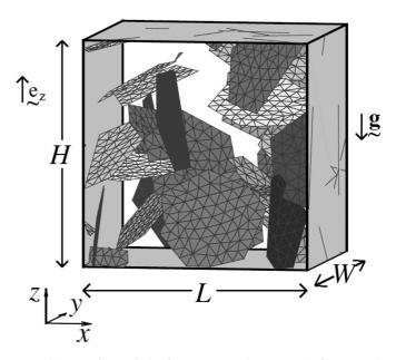
FIG. 1. An isotropic 3D fracture network composed of hexagonal fractures. The colors are only used to distinguish the various hexagons.
