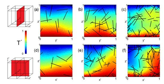
FIG. 9. The temperature field in two perpendicular vertical midplanes at steady state for (a), (d)  $\rho' = 2$ , (b), (e)  $\rho' = 6$ , and (c), (f)  $\rho' = 10$ . Data for  $\sigma' = 1$  and  $Ra_m = 41.5$ .
