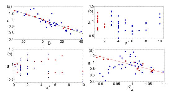
FIG. 17. The linear relation (29): *a* as a function of (a) *B*, (b)  $\rho'$ , (c) *b'*, and (d)  $K'_z = 2K_z/(K_x + K_y)$ . The solid line in (a) is a = 1 - b/100 and that in (d) is  $a = 3.4 - 2.5K'_z$ . Red dots and blue squares represent nonpercolating and percolating networks, respectively.
