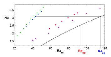
FIG. 6. The Nusselt number as a function of the matrix Rayleigh number  $\text{Ra}_m$ . The solid line is the interpolation (24b). Data for  $\rho' = 2\sigma' = 1$  (purple triangles),  $\rho' = 3$  and  $\sigma' = 5$  (green stars),  $\rho' = 4$  and  $\sigma' = 1$  (red dots), and  $\rho' = 7$  and  $\sigma' = 2$  (blue squares).
