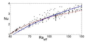
FIG. 11. The Nusselt number as a function of Ra<sub>eff</sub>. Black dots represent Nu with the FPM approach for  $0.1 \le \sigma' \le 10$ ,  $0.5 \le \rho' \le 10$ , and  $7 \le \text{Ra}_m \le 139$ . The dotted red line and solid blue line stand for two- and three-dimensional convection in a HPM.
