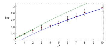
FIG. 14. The Nusselt number as a function of the dimensionless density of fractures,  $\rho'$ , for  $\sigma' = 1$  (red dots) and  $\operatorname{Ra}_m = 41.5$ . Dots represent the statistical average over 18 different networks with the same  $\rho'$ . Error bars represent the standard deviations. Solid green and dotted blue curves are the predictions for Nu deduced from Eqs. (24a) and (26a) and Eqs. (24b) and (26b), respectively, with solid and dotted lines in their range of validity.
