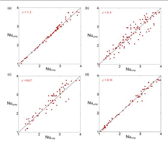
FIG. 13. The Nusselt number Nu<sub>HPM</sub> computed in a homogeneous porous medium as a function of the Nusselt number Nu<sub>FPM</sub> computed in the discrete fracture medium with the same effective permeability. One dot represents one realization, and the first bisector is added for clarity. Data for (a)  $\rho' = 1$  and 2, (b)  $\rho' = 3$  and 4, (c)  $\rho' = 5$ , 6, and 7, and (d)  $\rho' = 8$  and 10.
