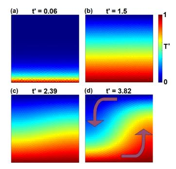
FIG. 2. Evolution of the temperature field in a vertical cross section of a pseudo-two-dimensional box  $(1 \times 1 \times 0.025)$ . Ra = 50,  $\delta'_M = 0.0167$ . (a) The simulation starts from a uniform temperature field. (b) A conductive temperature field is established. (c) Because of the overcritical Ra, the conductive temperature field is destabilized. (d) Steady-state 2D convection for Ra = 50.
