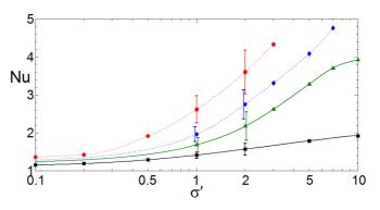
FIG. 8. The Nusselt number as a function of the dimensionless fracture transmissivity  $\sigma'$ . Data for  $\rho' = 8$  (red circles), 4 (blue diamonds and green triangles), and 1 (black squares);  $Ra_m = 41.5$ . Solid and dashed lines correspond to small and large Nu increments, respectively. The error bars correspond to  $\pm 2\sigma_d$ ,  $\sigma_d$  being the standard deviation observed over a set of 18 realizations (Fig. 10).
