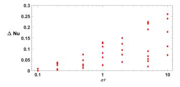
FIG. 15. The deviation  $\Delta \text{Nu} = |Nu_{\text{FPM}} - Nu_{\text{HPM}}|/Nu_{\text{FPM}}$  between fractured and homogeneous porous media with the same effective permeability as a function of the dimensionless transmissivity of fractures  $\sigma'$  for a density  $\rho' = 4$  and  $12 < \text{Ra}_m < 138$ . Each data point corresponds to one realization.
