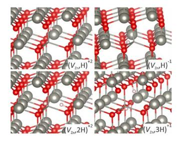
**Figure 4.** Structural models for the most stable atomic configurations of each of  $(V_{Zn}-H)$ ,  $(V_{Zn}-2H)$ , and  $(V_{Zn}-3H)$  defect complex. Large grey balls denote Zn atoms, small red balls denote oxygen atoms and small white balls denote hydrogen atoms. The Zn atom in front of the  $V_{Zn}$  was removed for the sake of clarity and only its bonds with the neighboring oxygen atoms are presented.
