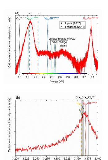
**Figure 5.** (a) Typical 5K cathodoluminescence spectrum of unintentionally doped ZnO NWs grown by CBD under standard conditions using the spontaneous growth approach. The insets represent the emission energy of transitions as inferred from DFT calculations in this work and in Refs. 21, 39. (b) Corresponding NBE emission region. The insets represent the emission energy of transitions as inferred from DFT calculations in this work and from experimental data in Refs. 34, 36.
