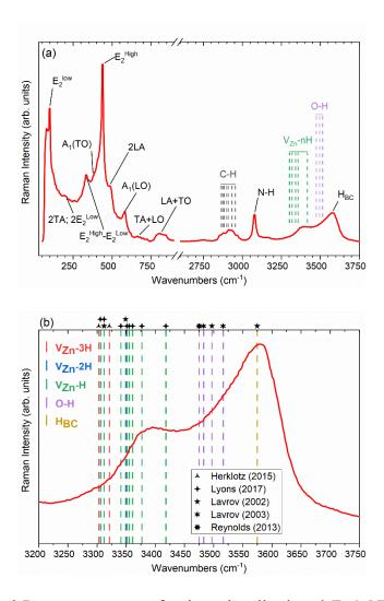
**Figure 6.** (a) Typical Raman spectrum of unintentionally doped ZnO NWs grown by CBD under standard conditions using the spontaneous growth approach. (b) Corresponding high wavenumber region. The insets represent the calculated and experimental vibrational frequencies from Raman and infrared absorption spectroscopy as inferred from Refs. 21, 33, 38, 104-105.
