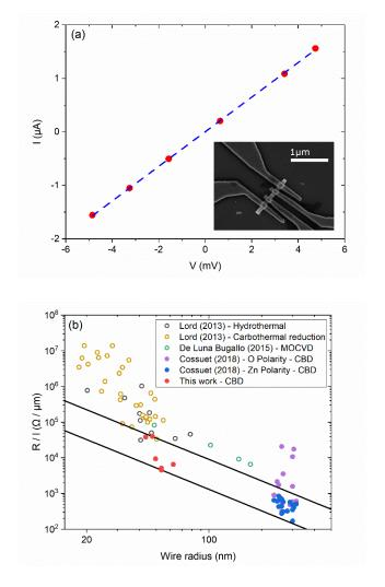
**Figure 2.** (a) Current-voltage (I-V) measurement using a four-point probe configuration on a single ZnO NW grown by CBD under standard conditions using the spontaneous growth approach. The inset is a top-view FESEM image of the single NW device in patterned metal contact configuration. The current is injected from the two outer contacts and the voltage drop is measured from the two inner contacts. (b) R/l versus r along with experimental data reported
