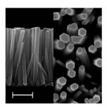
**Figure 1.** Cross-sectional- and top-view FESEM images of ZnO NWs grown by CBD under standard conditions using the spontaneous growth approach. The scale bar corresponds to 500 nm and 250 nm for the cross-sectional view and top-view images, respectively.
