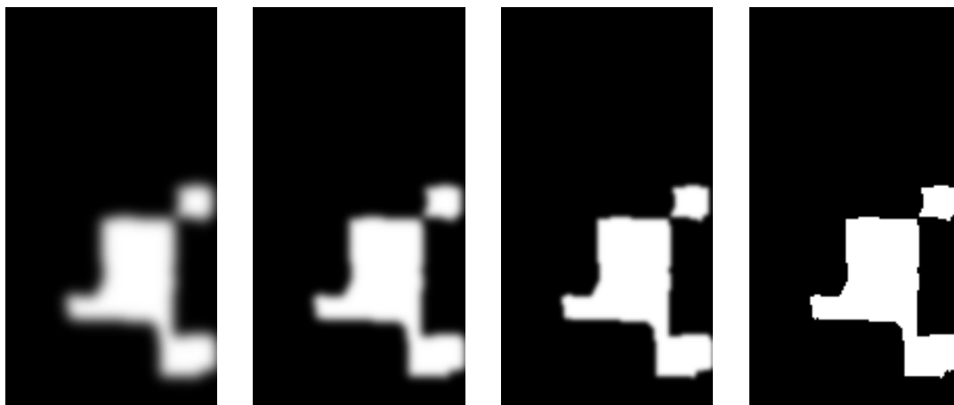
Figure 4: Blurred binarized thermograms used in the pyramidal approach, \sigma = [3, 2, 1, 0 px] from left to right
