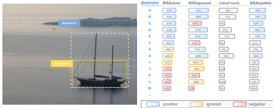
Fig. 2. Illustration of different anchor matching strategies for the boat image resorting to IoU_{anchor} (static), IoU_{regressed} ( Localize to Classify ) and IoU_{amplified} ( Classify to Localize ). Anchors A-M are predefined anchor boxes around the boat on the left side image, for simplicity, we only mark the position of the anchor F and the anchor H. Better viewed in colour.
