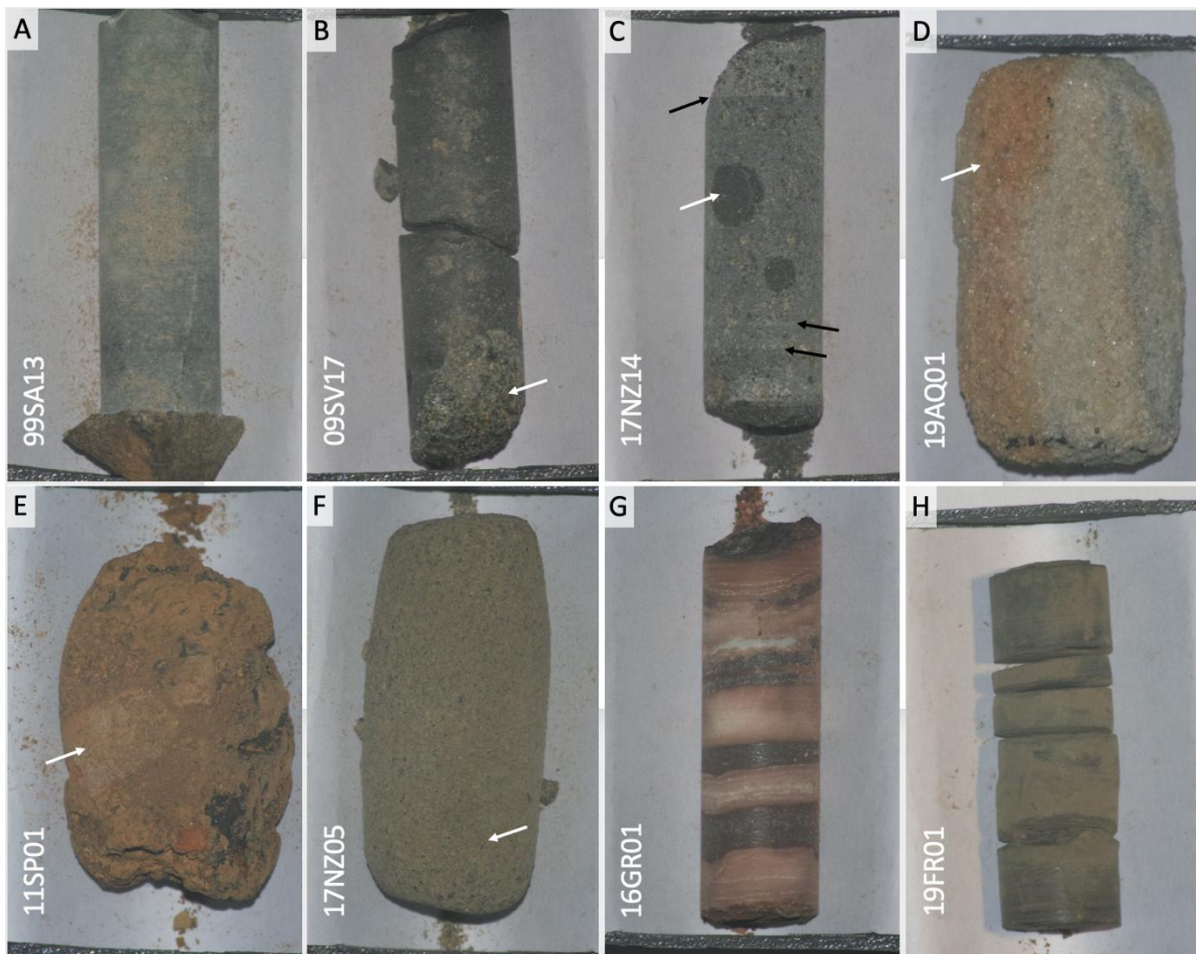
Fig. 4. Photographs (at maximal CLUPI resolution) of whole core samples, which are approximately 3 cm by 1cm in size. A) Sample 99SA13, metapelite with carbonate. B) Sample 09SV17, tholeiitic basalt with copious large olivine-rich xenoliths (white arrow). C) Sample 17NZ14, basalt-pyroxenite featuring large spherical
