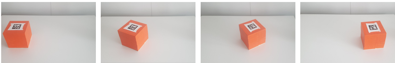
Fig. 2: Experimental setup to determine the physical properties of the cube. We considered two different scenes : in the first one, the unknown cube is sliding on the floor, starting with a given initial velocity v^0 ; in the second setup, the same cube collides with a second cube whose characteristics are known.
