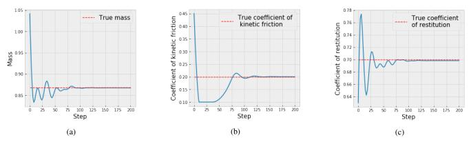
Fig. 6: The collision with an object, whose physical characteristics are known, allows to solve the ambiguity and retrieve the true parameters  $\mu$  and M simultaneously, which was not possible previously. In the same time, we are also able to find the value of the coefficient of restitution involved in the collision.
