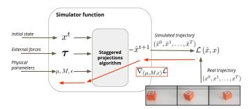
Fig. 1: Overview of our differentiable simulator. The differentiability of the simulator allows to integrate it into a larger learning architecture and infer physical parameters such as friction coefficients  $\mu$  and mass M of the objects, from real trajectories of these objects.
