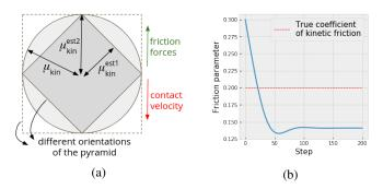
Fig. 5: Limitations of simulators approximating the friction cone with a pyramid [8],[11],[24],[26]. On Fig. 5a, the darker pyramid corresponds to the worst case, when the pyramid is rotated with an angle  $\pi/4$  with respect to the contact velocity. As predicted, Fig. 5b shows that the inferred value  $\mu_{\rm kin}^{\rm est1}$  converges towards  $0.141 = \mu_{\rm kin}/\sqrt{2}$ .
