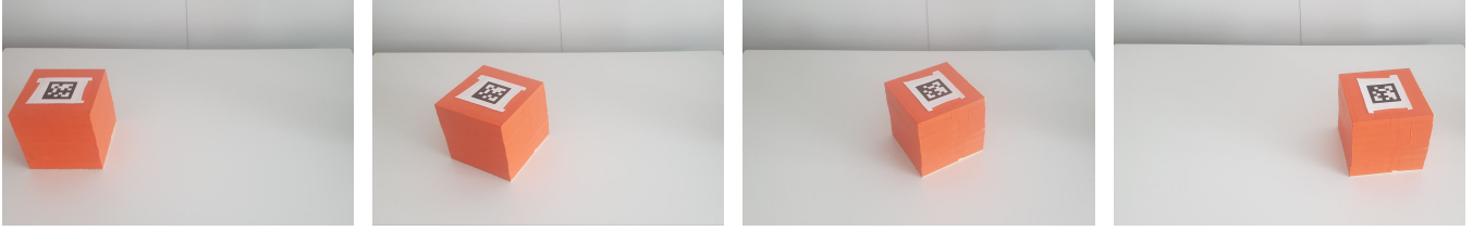
Fig. 2: Experimental setup to determine the physical properties of the yellow cube. We considered two different scenes : in the first one, the unknown cube is sliding on the floor, starting with a given initial velocity v^0 ; in the second setup, the same cube collides with a second cube whose characteristics are known.
