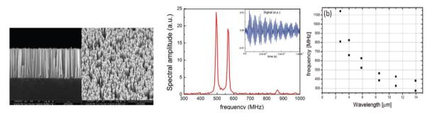
**Fig.2:** Left panel: MEB image of GaN NWs on n-doped Si(111) substrate. Center panel: Typical frequency spectrum of the laser-generated signal shown in the insert TGM acquired for the SAW wavelength  $\Lambda = 5.85 \mu m$ . Right panel: Experimental dispersion curves.
