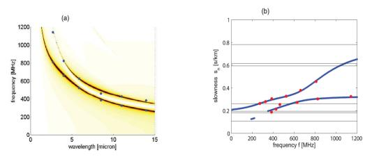
*Fig.3: Experimental points (bold dots), Green matrix element level-line images (a) and slowness dispersion curves (b).*
