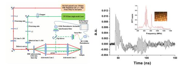
**Fig.1:** Scheme of the experimental setup (left panel) and typical temporal signal recorded obtained from a phononic cristal, made of Ni pillars, 400nm high and 50 $\mu$ m period, on a silicon substrate. This signal includes fast SAW oscillations of wavelength  $\Lambda$ =6.2 $\mu$ m (right panel).
