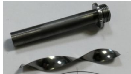
Figure 5: photograph of the transfer tube and associated helical chicane.
