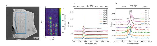
Figure 1: Activation of localized ensembles of SPEs on a hBN flake. (a) SEM image of a high-purity hBN flake of about  $15 \times 20 \mu m$  and 60 nm thickness. (b) Confocal map of the irradiated zone (blue rectangle in Fig. 1a) with eight irradiation spots (orange dashed lines). (c) and (d) Low-temperature spectra of the eight spots with two different spectral resolutions, showing a reproducible ZPL within 0.7 nm.
