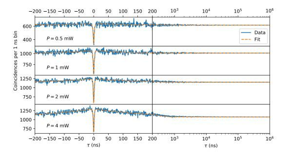
Figure 7:  $g^{(2)}(\tau)$  measured at four different powers. Left panel: linear scale around 0. Right panel: logarithmic scale for the time axis. The orange line is a fit with a function of the form  $g^{(2)}(\tau) = A - Be^{-|\tau|/t_1} + Ce^{-|\tau|/t_2}$
