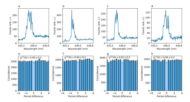
Figure 4: (a)-(d) Low-temperature PL spectra of four SPE ensembles and (e)-(f) corresponding RT secondorder correlation demonstrating some degree of antibunching. The orange dashed line denotes the classical limits. The value of  $g^{(2)}(0)$  is indicated above each histogram. The error bars represent 1 standard deviation as calculated from Poissonian statistics of the photon counting events.
