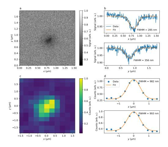
Figure 1: (a) SEM image of an irradiation on the  $SiO_2$  substrate. (b) Sum along x (upper panel) and y (lower panel) from which we estimate the beam dimensions. The orange lines are Gaussian fits of the data. (c) Room temperature photoluminescence confocal map of a SPE ensemble from an irradiation spot. (d) Cuts along x (upper pannel) and y (lower pannel) from which we extract the characteristic dimensions of the SPE ensemble.
