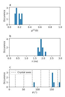
Figure 3: **Statistical dispersion of individual SPE properties.** (a)  $g^{(2)}(0)$  of 10 SPEs, showing single-photon emission. (b) Fluorescence lifetime  $\tau$  of the same 10 individual SPEs, with a mean value of 1.87 ns. (c) Polarization axis of the emission of 6 individual SPEs on the same flake, showing that most SPEs emit with a similar polarization direction.
