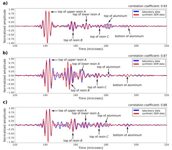
Figure 9. Comparison of zero-offset laboratory traces with the corresponding synthetic SEM results: a) trace A, b) trace B, c) trace C.
