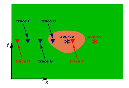
Figure 10. Location of the sources (asterisk) and receivers (triangles) associated to the two showcased offset experiments. The two data sets are denoted with red and blue colors, respectively.
