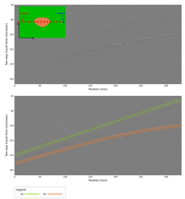
Figure 4. Cross section of the laboratory offset data set along the study line (i.e., common-shot gather) (top), and interpretation (bottom). Annotated events: (a) direct arrival and (b) reflection from the top of the upper resin A layer. The data were filtered between 250 and 650 kHz.
