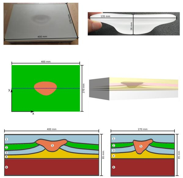
Figure 1. (a) The WAVES model after the assembly, (b) the glass dome placed inside, (c) top view of the WAVES model without the topmost layer, where the dashed blue line denotes the study line discussed in the paper, (d) illustration of the 3D geometry of the model, and (e and f) perpendicular vertical cross sections along the center lines of the model. The numbers denote the different materials whose properties are reported in Table 1.
