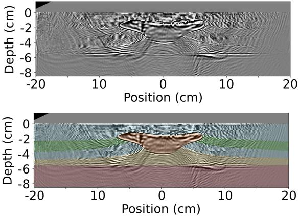
Figure 17. The impedance sensitivity kernel  $K_{\rho'}$  obtained with RTM. Top: the obtained kernel, bottom: the obtained kernel with an overlay of the original geometry (in color).
