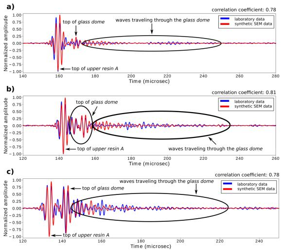
Figure 12. Comparison of offset laboratory traces with the corresponding synthetic SEM results: a) trace F, b) trace G, c) trace H.
