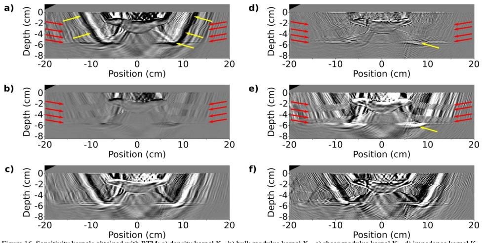
Figure 16. Sensitivity kernels obtained with RTM: a) density kernel  $K_{\rho}$ , b) bulk modulus kernel  $K_{\kappa}$ , c) shear modulus kernel  $K_{\mu}$ , d) impedance kernel  $K_{\rho'}$ , e) compressional-wave speed kernel  $K_{\alpha}$ , and f) shear-wave speed kernel  $K_{\beta}$ . Yellow arrows: artifacts, red arrows: known model discontinuities.
