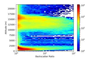
**Figure 3.** Distribution of Backscatter Ratio observations vs altitude. Data are 5 min averages of lidar vertical profiles, with 30 m vertical resolution. The colour codes the number of samples in each bin. Only data with BR>1.15 have bee reported.
