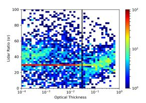
**Figure 9.** Distribution of Lidar Ratio (LR) vs optical thickness. The thick black line reports the optical thickness threshold value for SVC. The observations that accumulate along the line at LR=29 sr are those for which the inversion according to Young (1995) did not produce convergence to a result for LR. For these observation, LR was set at 29 sr by default.
