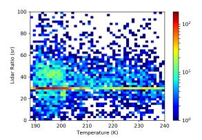
**Figure 11.** Distribution of Lidar Ratio (LR) vs mid cloud Temperature. The observations that accumulate along the line at LR=29 sr are those for which the inversion according to Young (1995) did not produce convergence to a result for LR. For these observation, LR was set at 29 sr by default.
