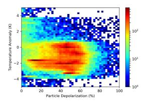
**Figure 13.** Distribution of particle depolarization observations vs temperature anomaly with respect to the average temperature profile as reported in the left panel of figure 2. Only data from clouds within 2500 m from the CPT are reported.
