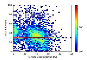
**Figure 10.** Distribution of Lidar Ratio (LR) vs Particle Depolarization. The observations that accumulate along the line at LR=29 sr are those for which the inversion according to Young (1995) did not produce convergence to a result for LR. For these observation, LR was set at 29 sr by default.
