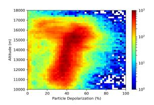
Figure 7. Distribution of particle depolarization vs altitude. Only datapoints with BR>1.15 are reported.
